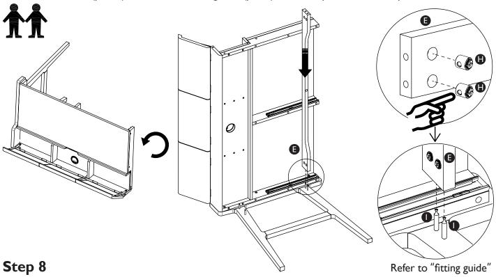
Use the allen key (part L) to insert spring washer (part J) and flat washer (part K) with bolt (part F) to secure front rail as shown below.
