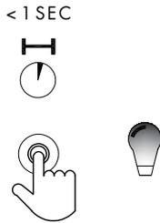
Quickly press the touch sensor to switch off the lamp
