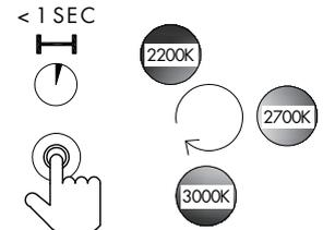
Quick tap on the touch sensor to change the color temperature of the lamp
