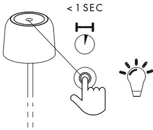
Quickly press the touch sensor to switch on the lamp
