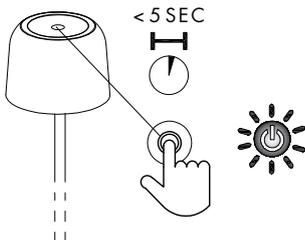
When the lamp is switched off, presslightly for 5 seconds until a steady blue LED lights up
