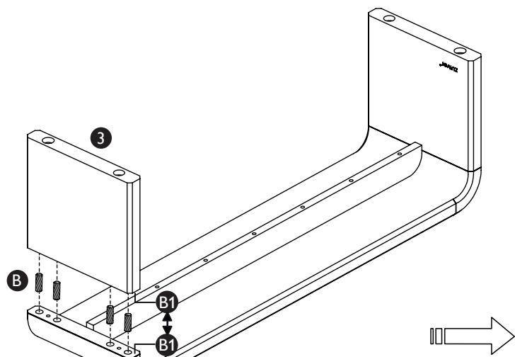
NOTE: legs are specific, refer to code B1 to locate the legs in the correct orientation.
