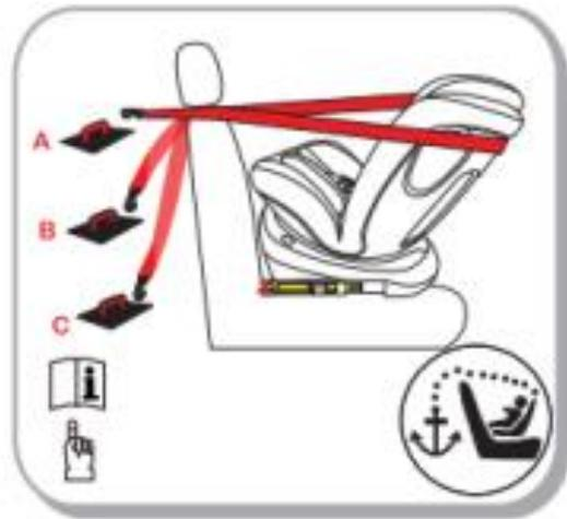
**Step7:** Pull the tether strap on another end back to tighten the top tether .
