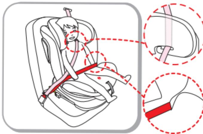
Step6: Insert diagonal belt and lab belt into the vehicle buckle hear "click" .Check the vehicle beltbuckle is correctly locked by pulling the seat belt -upwards.
