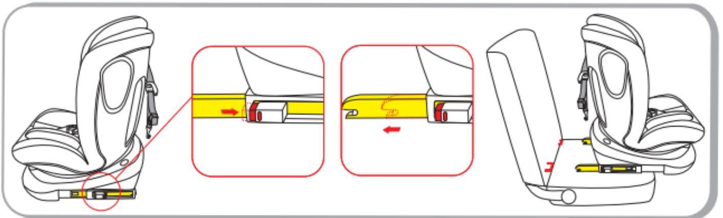
Step2: Push the ISOFIX connectors directly into the anchorages until heard an audible sound "click". Now the ISOFIX indicator of ISOFIX release button show green color .Ensure the child seat firmly pressed against the car seat's backrest.
