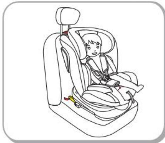
Step5. Pull out the vehicle belt, thread the belt tongue (incl. vehicle belt ) through one seat belt route slot to the rear and through the backrest, through the other seat belt route slot on the buckle side of the vehicle and allow it to lock in place .
