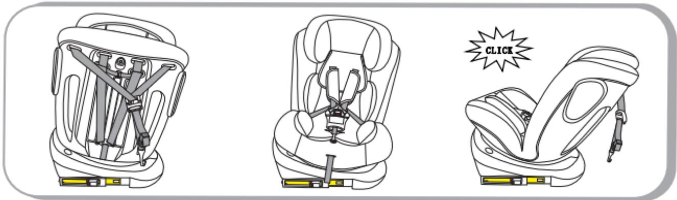
Important: Check to make sure the child seat is securely locked in the desired direction by shaking the seat body in clockwise direction or counter-clockwise direction .
