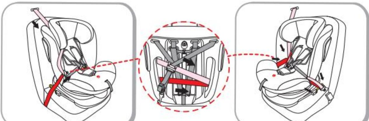
**Step6:** Insert diagonal belt and lap belt into the vehicle buckle hear "click" .Check the vehicle belt buckle is correctly locked by pulling the seat belt -upwards.
