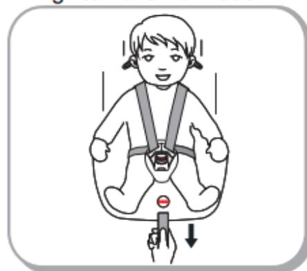
Pull the shoulder straps upwards to remove the slack from the lap sections of the harness then pull the adjuster strap until the harness is fully tightened.
