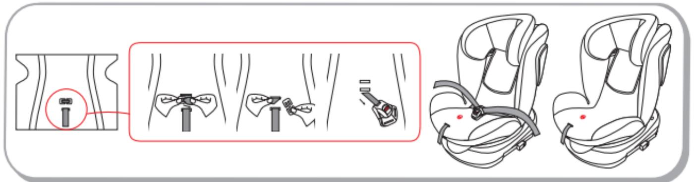
**Step5:** Adjust the child seat to incline position 1, pull the harness adjuster strap, now the car seat can be used without harness for children 15kg to 36 kg in weight (group II,III )
