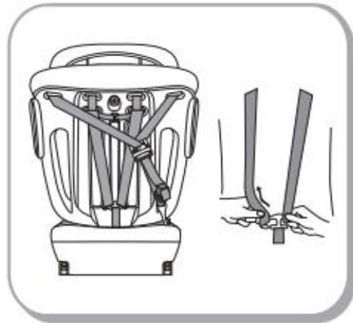
Step2:Pull shoulder straps through the shoulder strap slots from the front of the child seat. Pull the shoulder straps off the shoulder pads, now you can hide the shoulder pads behind the cover of the headrest .
