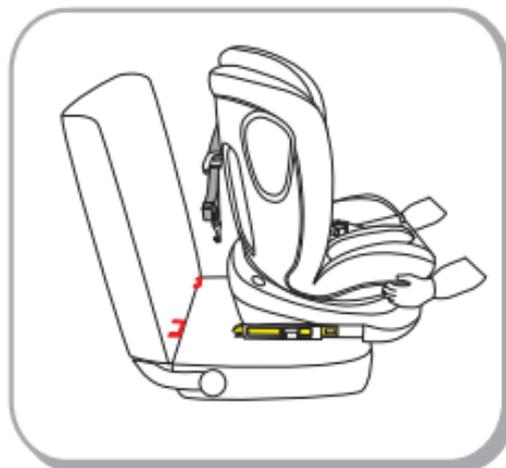
Step3: Grasp the seat body and base to check the seat if it is fastened tightly or shakes. If the seat shakes and the ISOFIX connectors are pulled out, please repeat the above steps and install it again. Release the incline handle once it is engaged in the desired direction until you hear a "click".
