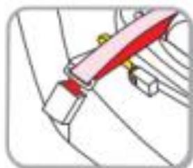
Make sure the seat belt has not become twisted. Also check that the cover is not impeding the movement or fit of the seat belt strap in any way .
