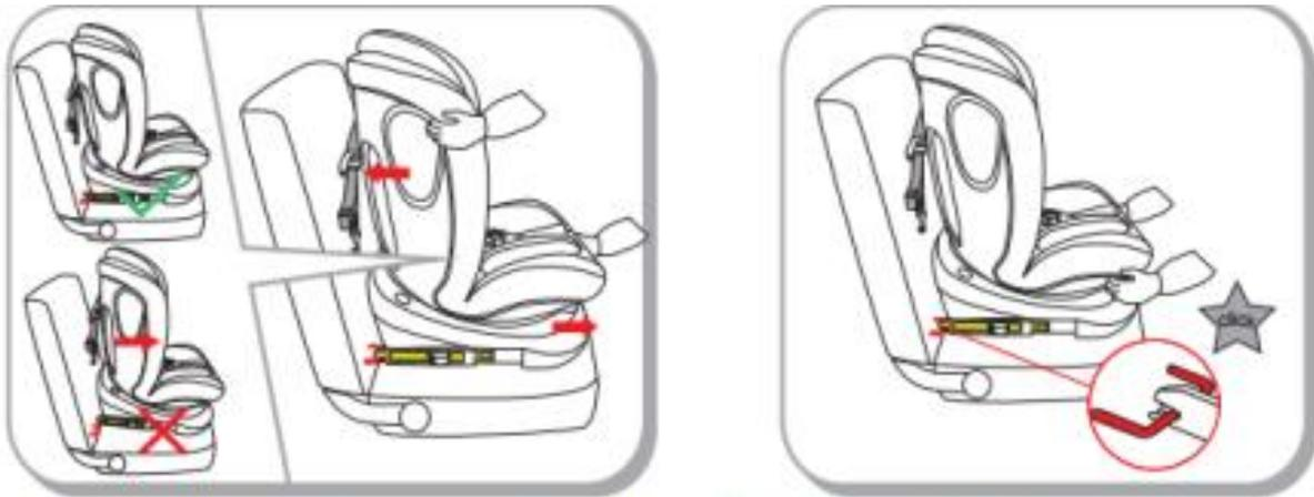
**Step4.** Press the rotation handle and rotate the body to the rearward facing direction. Release the rotation handle until you hear a "click". Pull or push the incline handle under the front of the seat to the rearward position, until you hear a "click"
