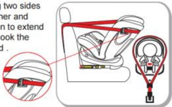
**Step6:** Hook the tether strap hook onto the user-ready anchorages. Check there maybe are 3 anchorages for the hook, please find one in your favor .
