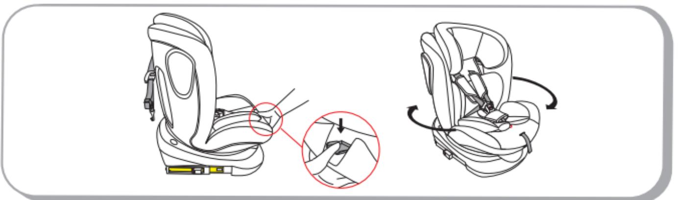
Release the incline handle once it is engaged in the desired direction until you hear a “click” .
