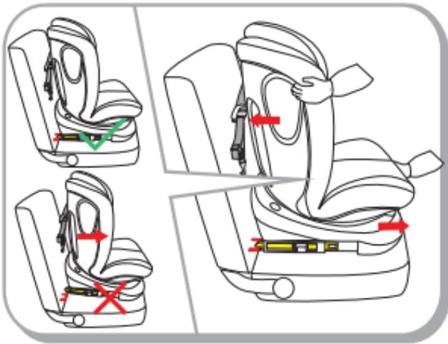
**Step4:** Grasp the seat body and base to check the seat if it is fastened tightly or shakes. If the seat shakes and the ISOFIX connectors are pulled out, please repeat the above steps and install it again .
