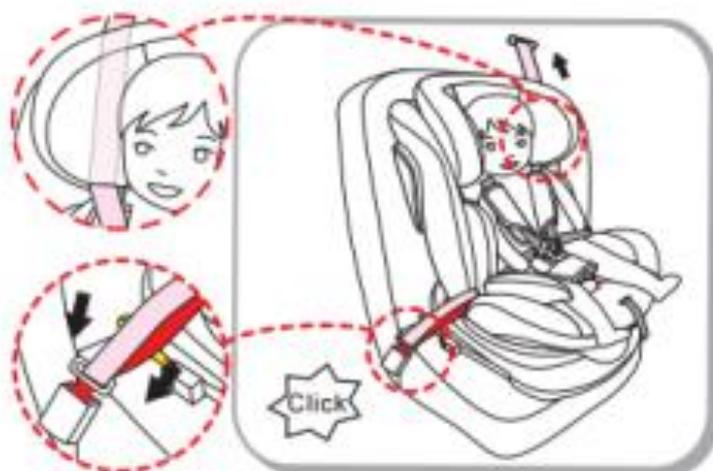
**Step7:** Check that the diagonal belt and lap belt have not become twisted and also check that the cover is not impeding the movement in any way.
