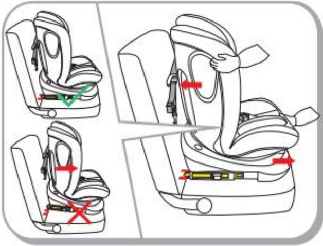
Step3: Grasp the seat body and base to check the seat if it is fastened tightly or shakes. If the seat shakes and the ISOFIX connectors are pulled out, please repeat the above steps and install it again .
