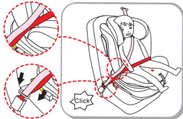
Step7: Check that the diagonal belt and lap belt have not become twisted and also check that the cover is not impeding the movement in any way.
