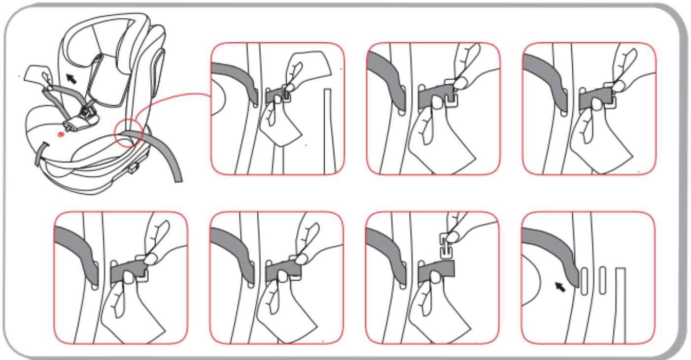
**Step4:** Slide the crotch strap off the belt locking clip as photos, now you remove the crotch pad ,crotch strap , buckle.
