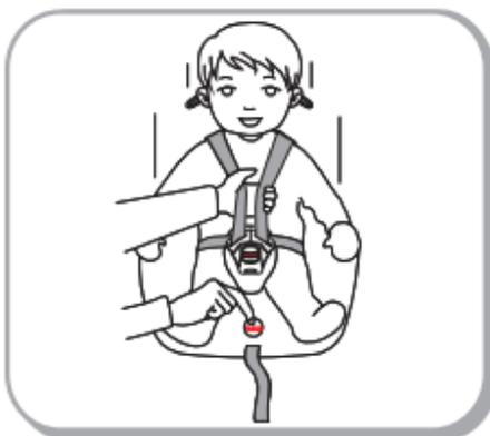
The harness is slackened by pressing the adjuster (under the seat cover) on the front of the seat.
