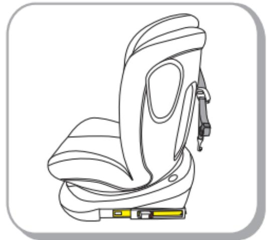
**Step2: Place the child seat on the car seat forward-facing and press the ISOFIX release button on both sides of the seat and push the ISOFIX connectors forward and make the ISOFIX connectors fully extend. This ensures that both hooks on the ISOFIX connectors are open ready to use, now the ISOFIX indicator of ISOFIX release button show red color.**
