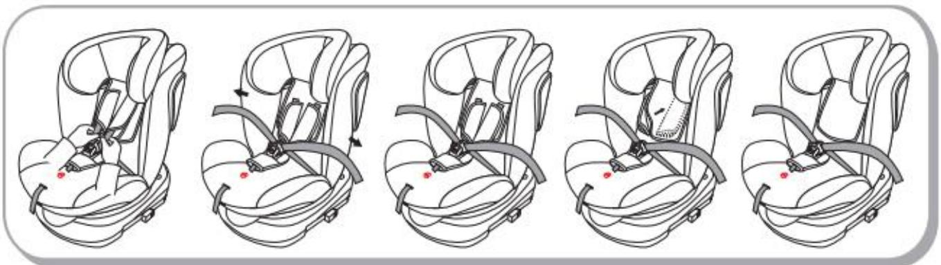
Step3:Slide the shoulder strap off the belt locking clip as photos, now you remove the shoulder straps.
