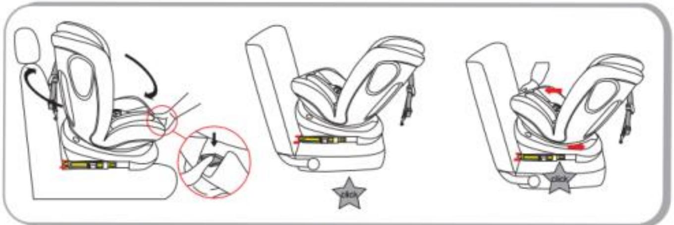
**Step5:** Slide the upper straps along two sides of the headrest, Pull out the top tether and press the tether strap release button to extend the strap until it is long enough to hook the user-ready tether anchorage behind .
