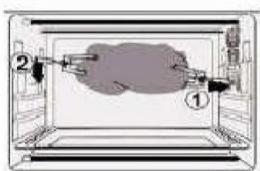
Insert the rotisserie forks in the rotisserie orifice and then place the drip pan under the rotisserie
