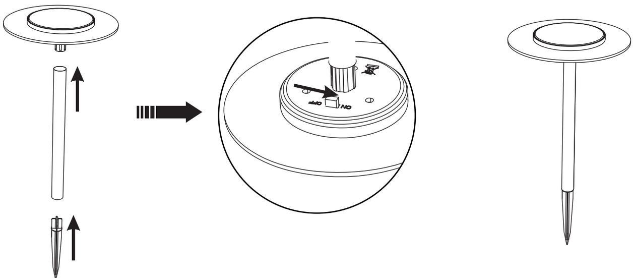
1. Install the light head, pole and spike.
