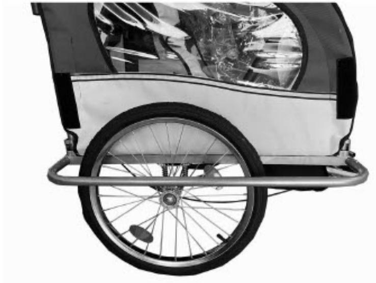
Rails are an additional protection against the wheel sliding out, the installation of these is necessary!
