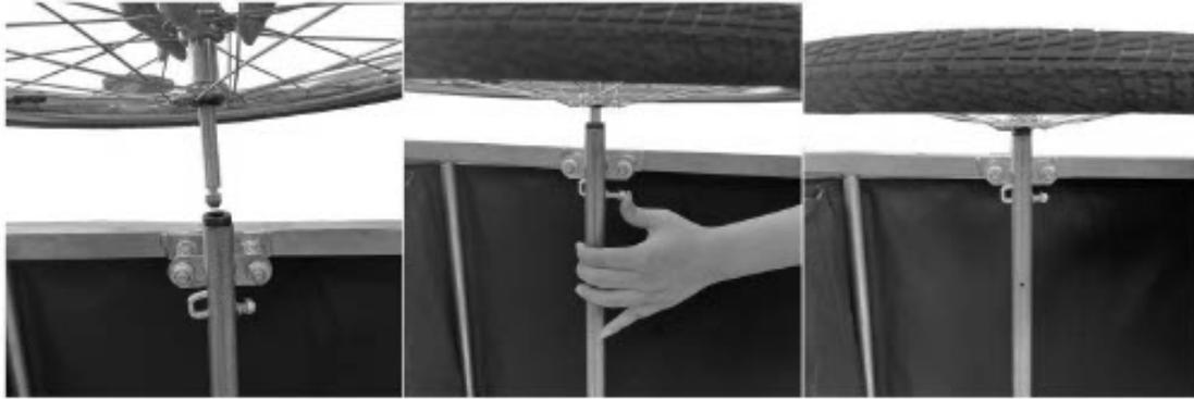
f) Place the metal brackets to protect the wheels so that the latches in the frame secure the wheels.
