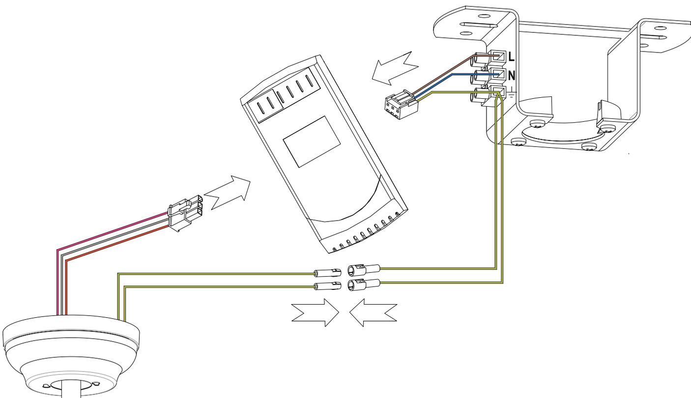
Check that all electrical connections have been correctly made and that the receiver and the wires are properly stored in the hanger bracket.
