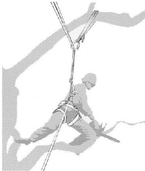
Example of deflection of the main rope via an additional suspension device.
