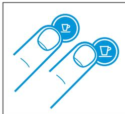
5. To enter the descaling mode, while the machine is turned on, press both the Espresso and Lungo buttons for 3 seconds.
