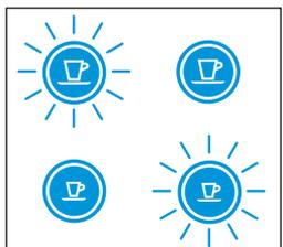
Both LEDs blink alternately.
