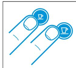
To turn the machine off before automatic Power Off mode, press both the Espresso and Lungo buttons simultaneously.
