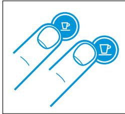
10. To exit the descaling mode, press both the Espresso and Lungo buttons for 3 seconds.
