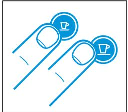
1. To enter the emptying mode, press both the Espresso and Lungo buttons to turn the machine off.
