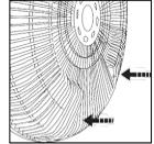
4. Replace and screw the lock ring of rear grill (6) back onto the motor block (11) to secure the rear grill assembly; turn clockwise. Make sure to tighten the ring properly.
