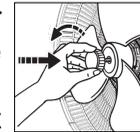
6. Properly align the arrows on the top of the front grill (2) with the rear grill (7). Push the front grill clips into the rear grill until you hear a snap for each clip.
