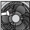
To remove dust inside and on the grilles, use a vacuum cleaner with a suitable nozzle. Do not disassemble the fan to clean it.
