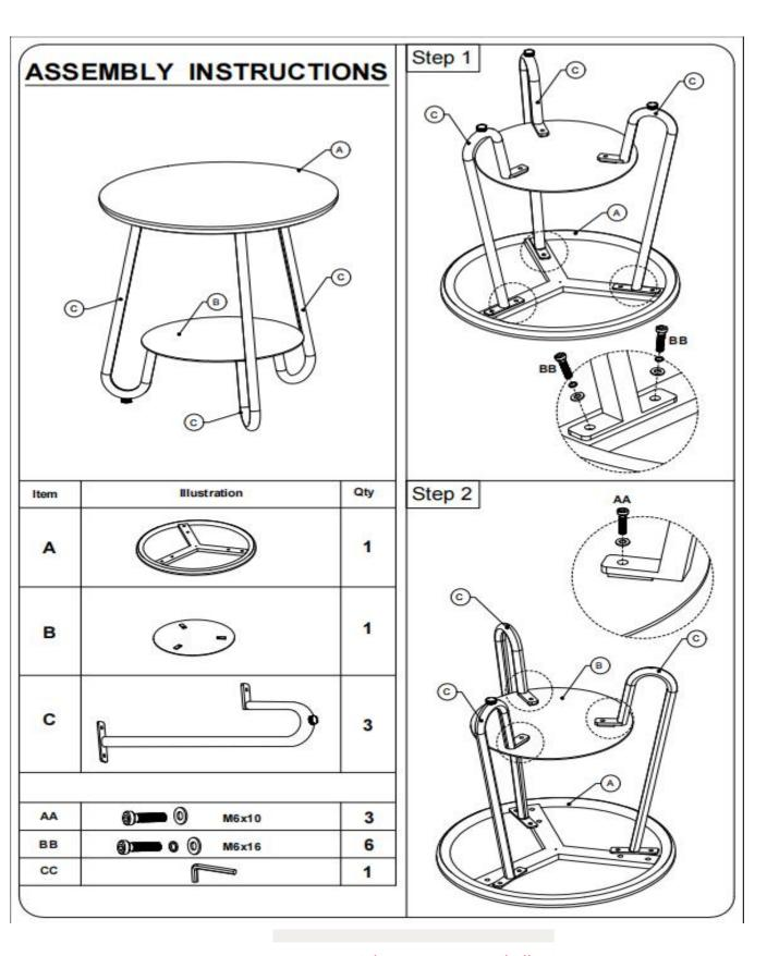
Do not tighten screws until all screws have been assembled!
