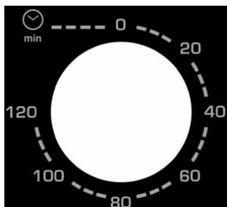
Set the timer to the cooking time (in minutes) depending on the dish you are cooking by turning it clockwise. The indicator light allows you to ensure the orderly functioning of the heating elements. The oven will turn off automatically at the end of the selected time and a bell will ring. The oven can be turned off manually during cooking by turning the timer anti-clockwise to the "0" position.
