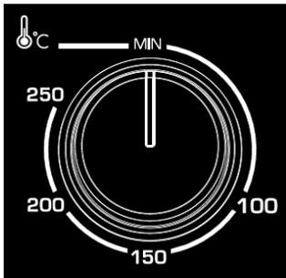
Set the "Temperature Control" by turning the knob clockwise to the suitable temperature for the dish you are cooking. (Temperature Control between 70°C and 250°C)
