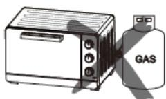
During the use, do not position the oven near a gas burner or any other heat source. Doing this could affect the temperature control.
