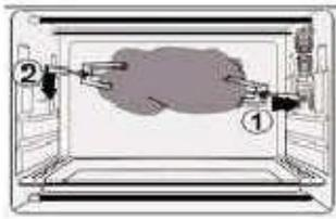
Fit the rotisserie forks in the rotisserie holes and then install the drip pan under the rotisserie
