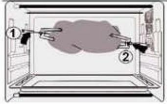
Use the rotisserie handle to remove the rotisserie forks from the rotisserie tray and then remove it from the rotisserie hole
