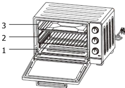
There are 3 different positions for the tray which can adjust according to the dish you are cooking. For example, when you are cooking a gratin and you want to have the top part cooked the most, use the third position. To roast a chicken, use the first or the second position.
