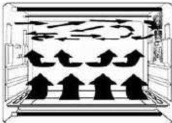
Thanks to the fan function on the side of the cavity, the hot air circulates in the entirety of the oven, so the heat is better distributed and the cook is more uniform.
