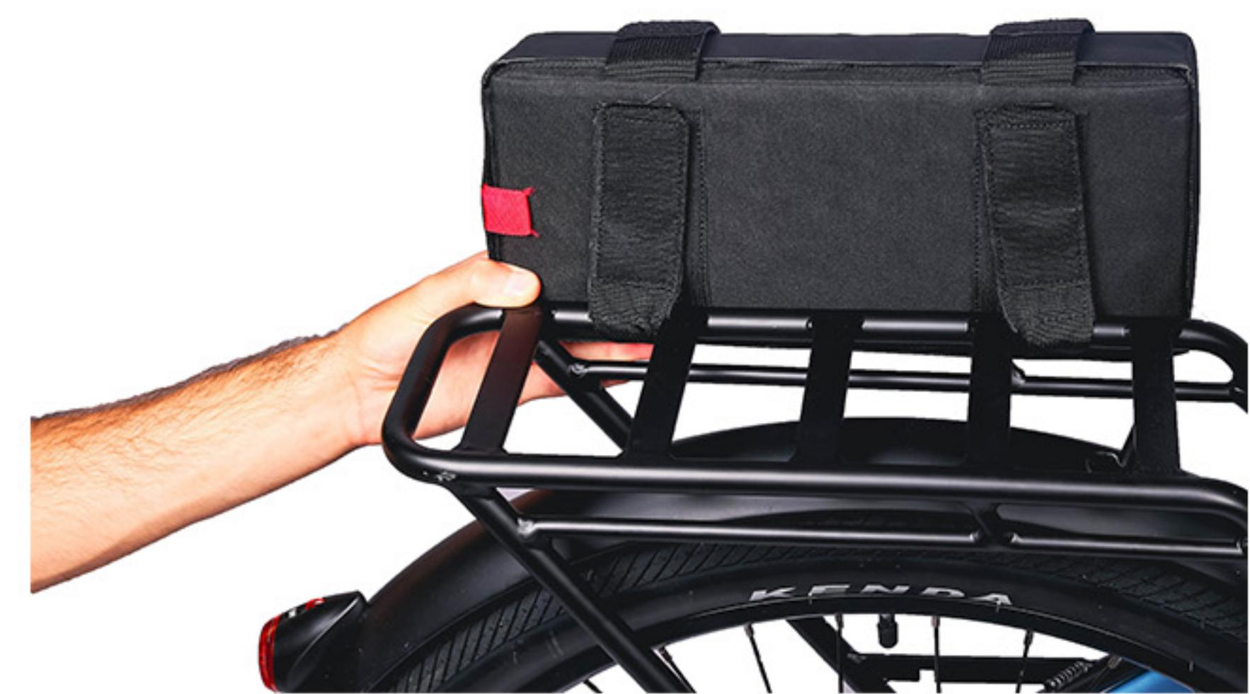
5. Place the support on the luggage rack and attach the top strap under.
