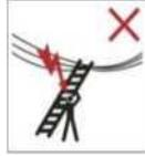
Identify electrical hazards in the work area, such as overhead lines or other exposed electrical equipment and do not use the ladder where electrical hazards occur.
